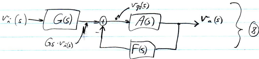
$$\left. \begin{aligned} (8) \text{ using Mason's gain formula} \\ \text{OR} \\ (7) \text{ using algebra} \end{aligned} \right\} \Rightarrow A_v(s) = G(s) \frac{A(s)}{1 + A(s)F(s)} \quad (9)$$
