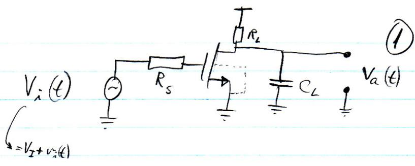
( $R_L$  &  $R_s$  often from active circuits, not actual resistors)
