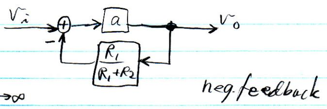
$$A = \frac{a}{1 + a \left( \frac{R_1}{R_1 + R_2} \right)} \rightarrow 1 + \frac{R_2}{R_1} \text{ as } a \rightarrow \infty$$
