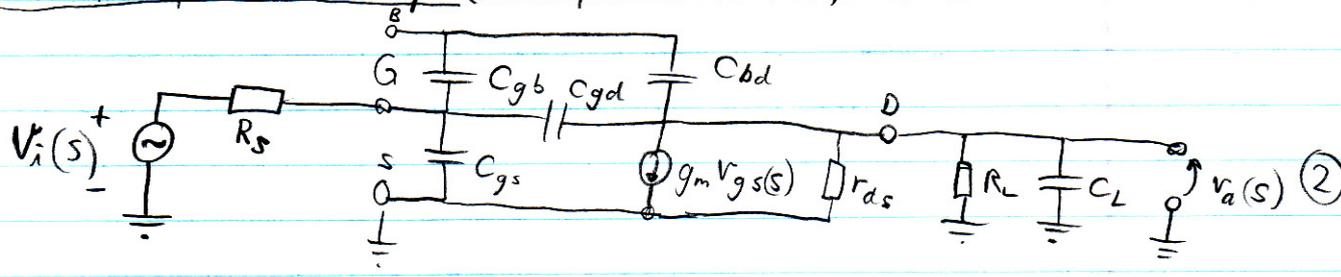
$$\left. \begin{aligned} v_{gs}(s) &= -F(s) \cdot v_a(s) + G(s) v_i(s) \\ v_a(s) &= A(s) \cdot v_{gs}(s) \end{aligned} \right\} \textcircled{7}$$
