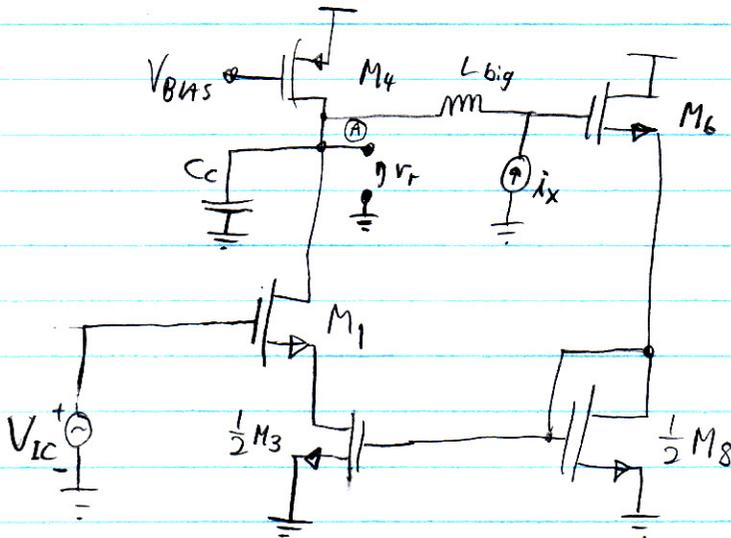
( $L_{big} \Rightarrow$  zero-freq voltages at two terminals of  $L_{big}$  are same, but  $L_{big}$  blocks non-zero frequency components)
