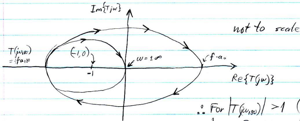
$\therefore$  For  $|T(j\omega_{180})| > 1$  (the case shown) have 2 c.w. encirclements, but  $T(s)$  has no RHP poles
