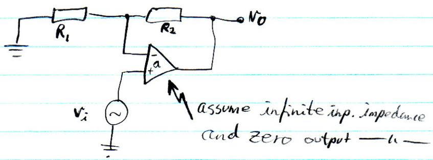
$$v_o = a \left[ v_i - \frac{R_1}{R_1 + R_2} v_o \right]$$
