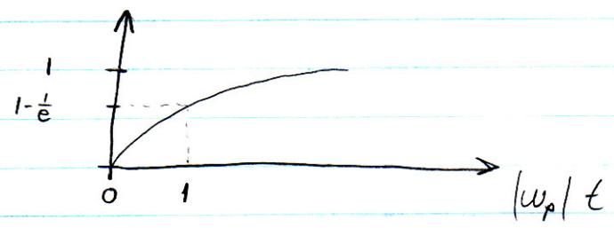
$$\mathcal{L}^{-1}\left\{\frac{1}{s} \cdot \frac{\omega_{op}^2}{s^2 + s(2\zeta_s \omega_{op}) + \omega_{op}^2}\right\} = u(t) \cdot \left[1 - \frac{1}{\sqrt{1-\zeta_s^2}} e^{-\zeta_s \omega_{op} t} \cdot \sin(\omega_{op} \sqrt{1-\zeta_s^2} \cdot t + \theta)\right]$$
