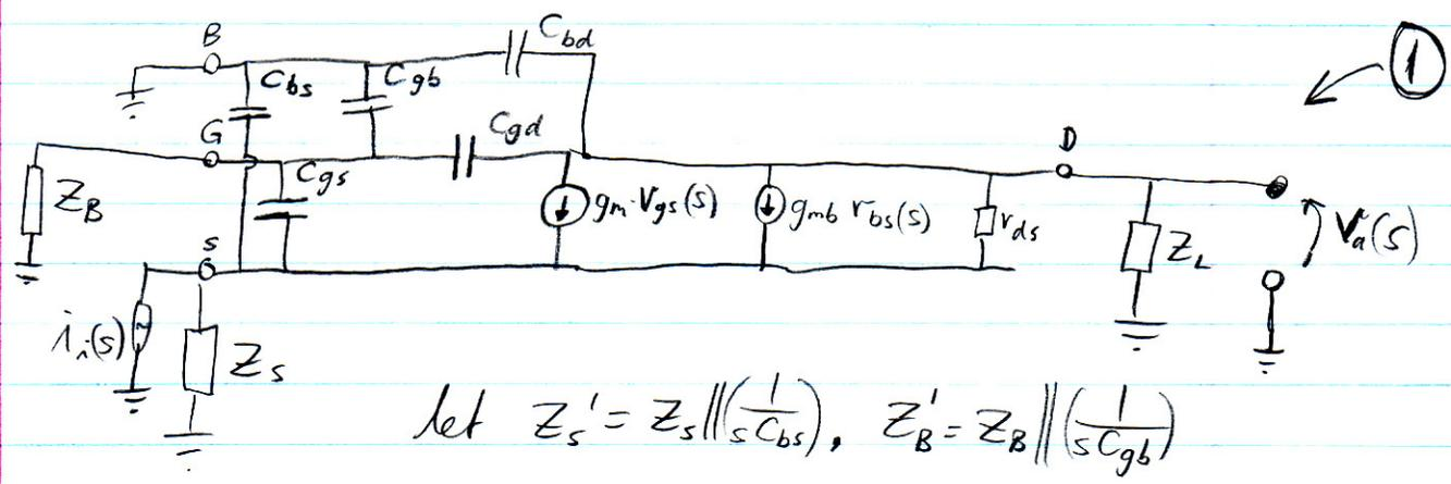
let  $Z'_s = Z_s \parallel \left( \frac{1}{s C_{bs}} \right)$ ,  $Z'_B = Z_B \parallel \left( \frac{1}{s C_{gb}} \right)$
