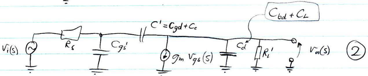
Last time: hard work gave us  $p_1 \approx \frac{-1}{(C_d + C')R_L' + (C_{gs}' + C)R_s + g_m R_L' R_s C'}$  (3)
