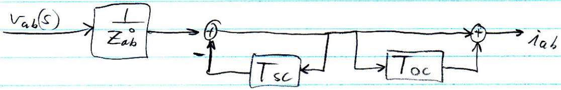
∴  $T_{sc}$  also arises from a feedback path within the circuit
