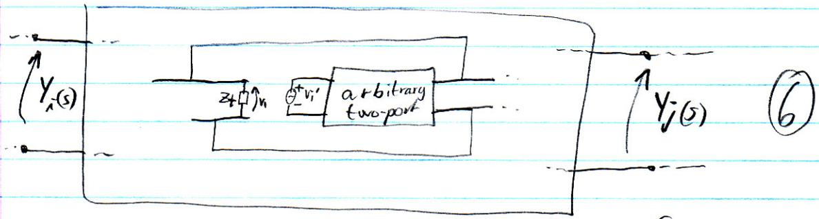
where  $v_i' = \alpha \cdot v_i$ , with  $\alpha \equiv 1$ ,  $Z_f \equiv \frac{v_i(s)}{i_i(s)}$  (input imp. of two-port depends on loading of  $Y_i(s)$  &  $Y_j(s)$  ports)
