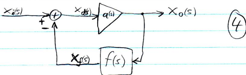
$a(s) \equiv$  "open loop gain",  $f(s) \equiv$  "feedback factor"
