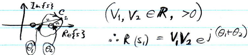
As  $C$  is traversed:  $\left\{ \begin{array}{l} \text{net change in } \theta_1 \text{ is } 0 \\ \text{net change in } \theta_2 \text{ is } -2\pi \end{array} \right.$
