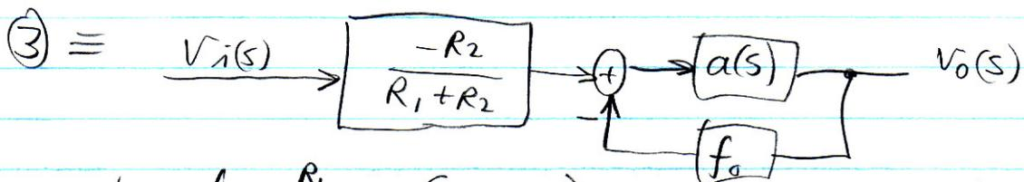
where  $f_0 = \frac{R_1}{R_1 + R_2}$  ( $0 < f_0 < 1$ )
