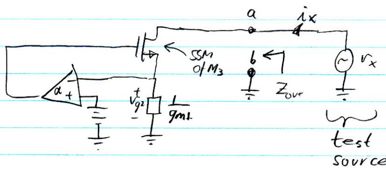
If  $v_x$  increases,  $i_x$  increases  $\Rightarrow v_{g2}$  increases
