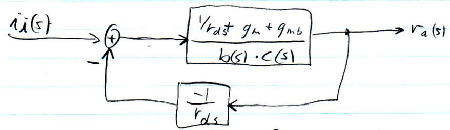
Now, MGF gives  $G(s) \Big|_{|Z_B|=0} = \frac{\left( \frac{1}{r_{ds}} + g_m + g_{mb} \right)}{b(s) \cdot c(s)} \cdot \frac{1}{1 - \frac{1}{r_{ds}} \left[ \frac{\left( \frac{1}{r_{ds}} + g_m + g_{mb} \right)}{b(s) \cdot c(s)} \right]}$
