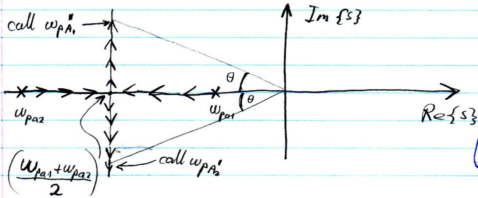
$$\frac{a(s)}{1+f \cdot a(s)} = \frac{a_0 \cdot \omega_{pa1} \cdot \omega_{pa2}}{s^2 - (\omega_{pa1} + \omega_{pa2}) \cdot s + (1+a_0 \cdot f) \cdot \omega_{pa1} \omega_{pa2}}$$
