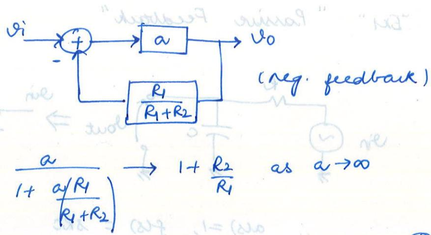
$$A = \frac{a}{1 + \frac{a/R_1}{R_1+R_2}} \rightarrow 1 + \frac{R_2}{R_1} \text{ as } a \rightarrow \infty$$
