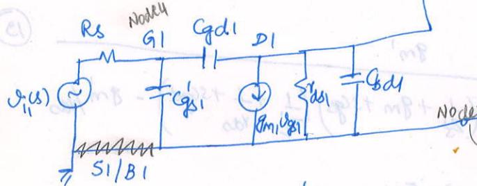
where  $C_{gsi} = C_{gsi} + C_{gbi}$ ,  $C_3 = C_{gs3} + C_{gd3}$ .
