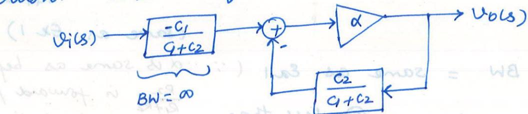
$$\text{Ans} \quad \text{with } \begin{cases} a = \alpha \\ f = \frac{C_2}{C_1 + C_2} \end{cases} \Rightarrow f = \text{const. (EIR)}$$
