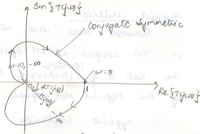
$\Rightarrow$  No encirclements of  $(-1, 0)$  ( $T(s)$  has no RHP poles by inspection)
