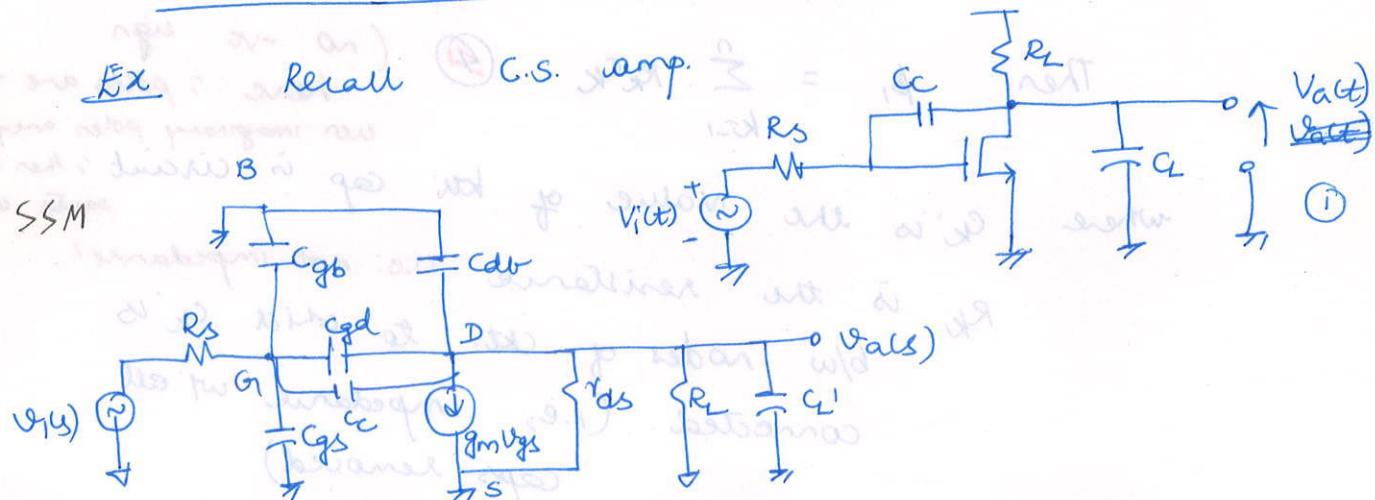
$$= \frac{R_s}{R_s + G} \frac{C' = C_{gd} + C_d}{C' + C_{gs}} \frac{D}{D + S}$$
