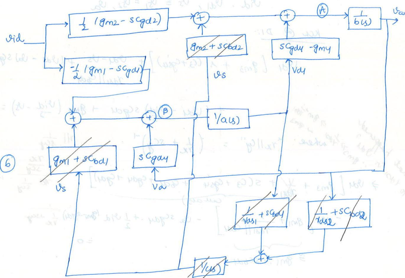
$$\text{Let } P_1, P_2, \dots \text{ be the poles of } A(s) = \frac{v_{os}}{v_{id}} \text{ w/ } |P_1| \leq |P_2| \leq \dots$$
