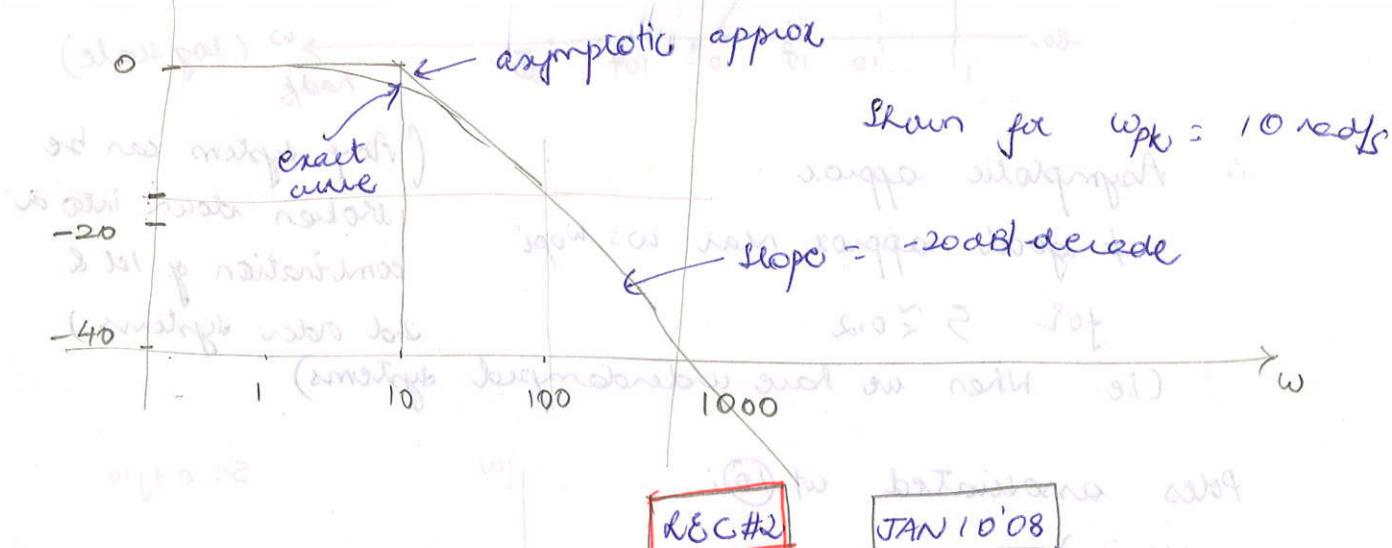
Recall ⑩ :  $\sum_{\text{complex pole pairs}} 10 \log \left[ \left( 1 - \frac{\omega^2}{\omega_{\text{op}}^2} \right)^2 + 4 \frac{\xi_p^2}{\omega_{\text{op}}^2} \omega^2 \right]$
