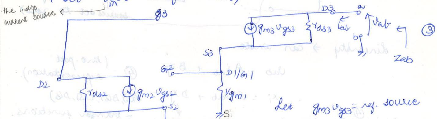
$$\text{Inspection of } (3) \Rightarrow Z_{ab} = r_{ds3} + \frac{1}{g_m} \approx r_{ds3}$$
