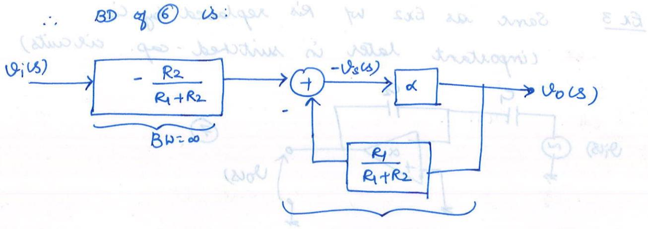
$$\Rightarrow \text{① w/ } \alpha = \alpha \text{ & } f = \frac{R_4}{R_1+R_2}$$
