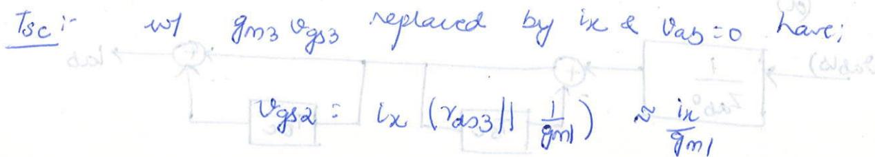
$$v_{gs2} = i_x \left( r_{dss3} \parallel \frac{1}{g_{m1}} \right) \approx \frac{i_x}{g_{m1}}$$
