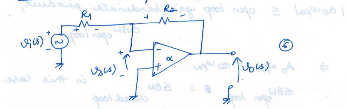
$$V_o(s) = \alpha(s) [-V_s(s)] \quad \text{(from notes)} \\ V_s(s) = (V_i(s))_{\text{new}} = R_1 \left[ \frac{(V_i(s) - V_o(s))}{R_1 + R_2} \right]$$
