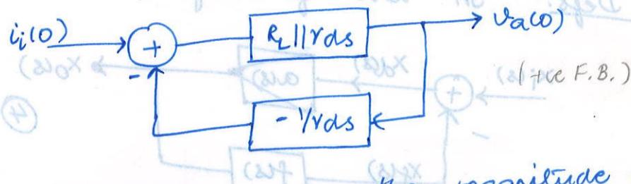
Note: In Ex 1, feedback reduces the magnitude of  $x_0 \Rightarrow$  "negative feedback"  $\equiv (a(s) < 1)$
